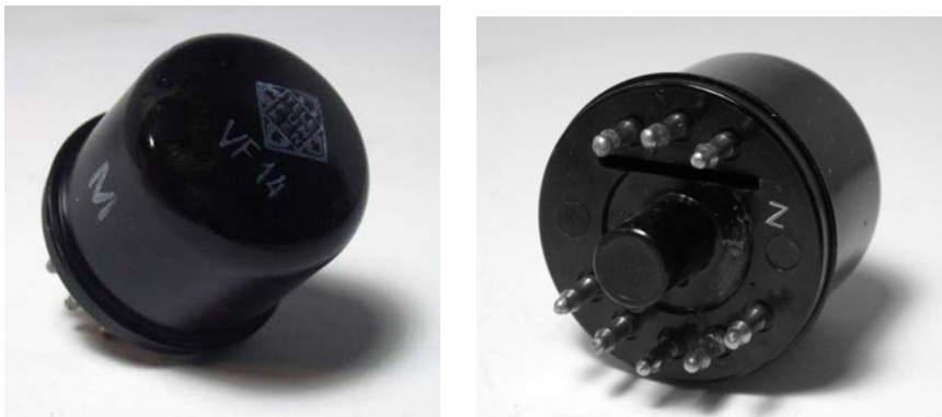
Figure 36 - The VF14 valve used in the impedance converter of the U47
