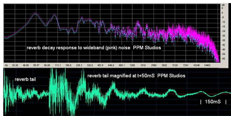
**Figure 17 - Using the DAW as an acoustic measurement system**
