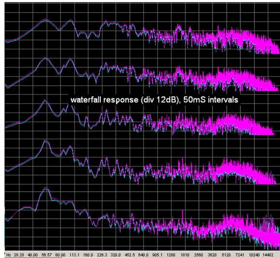
**Figure 18 - Fourier analysis performed over 50mS intervals during the reverb tail**
