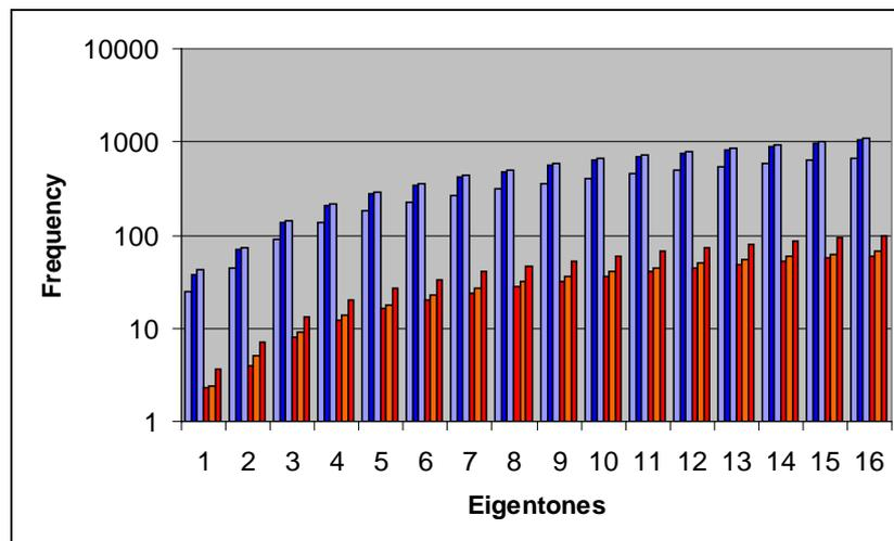
**Figure 16 - First sixteen eigentone frequencies for a small room (long bars) and a large room (short bars)**
